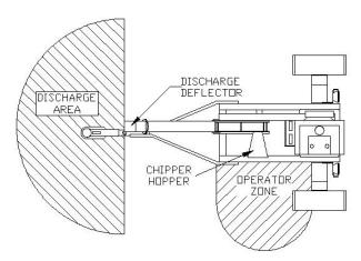
THE EXACT AREA OF DISCHARGE WILL BE DETERMINED BY THE DIRECTION OF THE DISCHARGE CHUTE AND THE ANGLE OF THE DEFLECTOR.
